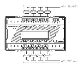
After the power supply is connected correctly, the LCD should display "Press Addressing Key to be addressed", otherwise it will show "OFF LINE"
