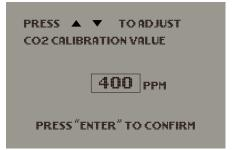
After selecting either **TEMP**, **HUMID** or **CO2**, users can adjust the calibration value by presse , the press to confirm.
