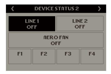
The DEVICE STATUS 2 indicates lighting status, Aerofan status, and/or EC fan status. This page indicates the 2 channel LED lighting (LINE 1 & LINE 2) status, Fan (F1-F4) status and AeroFan status.
