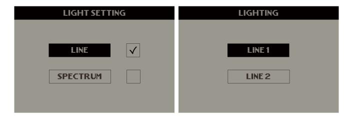
After pressing **ENTER** on the **Light Setting**, the screen will display the Line tab and Spectrum tab. Use the and arrows to select between the Line tab and Spectrum tab, and press **ENTER** to navigate to the page where you can make changes to the selected option.
