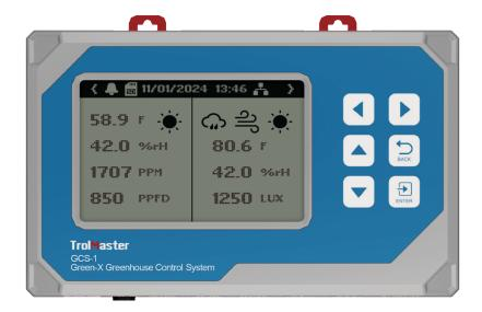
When you power up the GCS-1 for the first time, the homepage will display on the LCD. Use the "LEFT" and "RIGHT" arrows to switch between pages: climate data, nutrients and growing medium data, device status, and alarm notifications. Each page contains specific information about the GCS-1, which continuously monitors climate conditions and nutrient levels in real-time.
