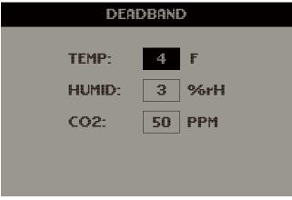
• **DeadBand:** You can set your deadband setpoints that will be used with your connected device modules. The deadband settings determine the temperature or humidity level that each module will turn on, and turn off again.
