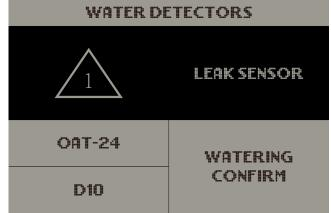
• Water Detectors: This page will show you the status of the optional Water Detectors. Here you can select one of two modes for the Water Detectors, Leak sensor or water confirmation sensor.
