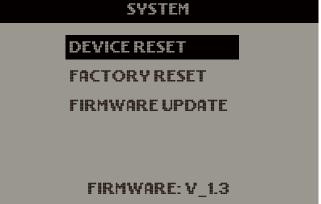
• System Reset: There are three options to choose from within the System Reset menu. Device Reset allows the user to reset ONLY the device module addressing. The Factory Reset can be used to resolve some major problems within the controller, or if the user just wants to return the unit to factory settings. You can also update the GCS-1 internal firmware by selecting Firmware update.
