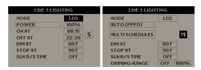
On the Line 1 / Line 2 settings, you can make changes to the light schedules. Use the and volutions to navigate the options on this page and press **ENTER** on an item to change it. When you see the item blinking, you can switch between the selections using the and volume. When you have selected your item, press **ENTER** again to confirm the selection and make changes to different settings below:
