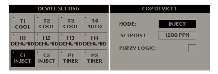
When you open the Devices page, you can select what each of your connected device modules will be controlling. You have 4 device slots available each for temperature T1,T2,T3,T4, humidity H1,H2,H3,H4; and 2 device slots available each for CO2 C1 & C2, programmable timer P1 & P2.
