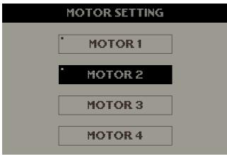
The Motor Setting page on the GCS-1 controller allows you to schedule motor operations to control curtains based on specific environmental conditions.
