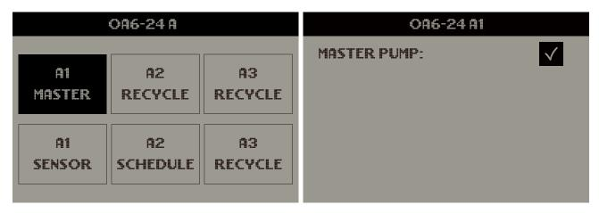
After selecting the **A1 SENSOR** tab, you will access the page where you can check the types and settings of your irrigation devices. When you click on the **A1 SENSOR** settings, you will find the master pump settings available for configuration.
