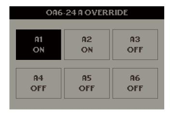
This is Irrigation Devices status, press **ENTER** to select irrigation device for override, user can either choose **ON** and **OFF**.
