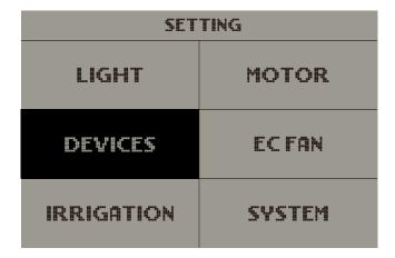
The Devices tab is where you will set up your climate control devices. With the use of our plug-in DS modules, you can connect and control the devices via the controller. TrolMaster's Green-X can control multiple device modules.
