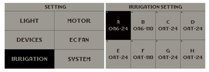
After pressing **ENTER** on the **IRRIGATION** tab, you will access the page where you can configure the settings for the irrigation devices. There are eight hubs available, allowing users to select either **Trolmaster's 6 Outputs 24V Control Board (OA6-24)** or the **110V Control Board (OA6-110)**. You can set up to a maximum of eight hubs.
