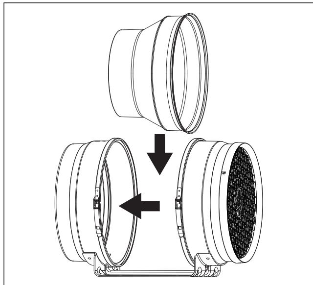
2. Insert the Air Booster into the fan cover, at the open end right opposite the cover.
