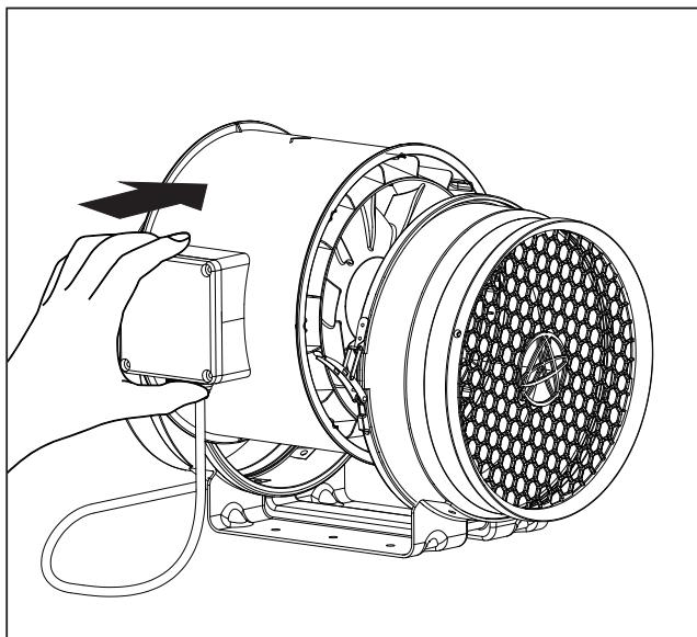
3. Reinstall the fan body back in the frame.
