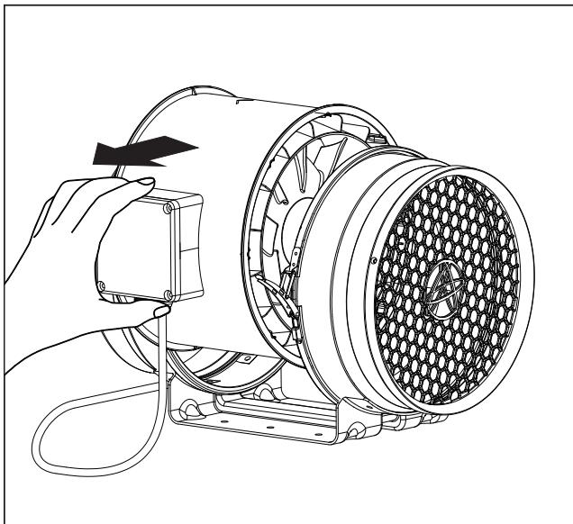
1. Unlock the clasps, release the fan body from the frame.
